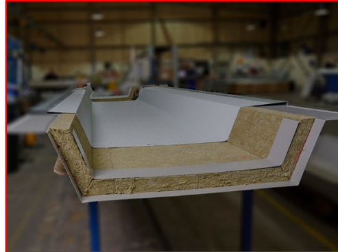
Figure 4: Manufacture of insulated membrane lined valley gutter
