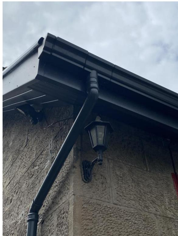
The Traditional Moulded Ogee bolted gutter system is manufactured to BS 8530, the original design standard for cast iron, and as such fully replicates the traditional look. The 125mm gutter has a flow-rate of 2.21 litres per second (l/s) and an effective roof area of 105m<sup>2</sup> per 63mm downpipe when fitted in an end outlet configuration.
