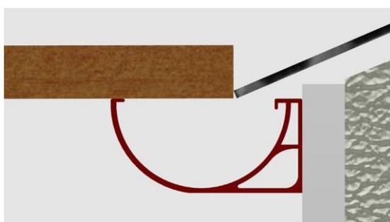
*Use a spirit level against the lowest point of the roof tile to determine the position of the fascia bracket*
