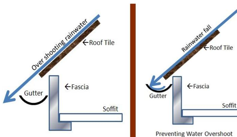
BS 5534:2014 (*Slating and tiling for pitched roofs*) states that roof tiling should project a minimum of 50mm from the vertical face of the fascia board. The projection should align with the centre line of the gutter and therefore this will establish the minimum width of gutter. However, there is no guidance as to the height of the gutter relative to the roof edge.
