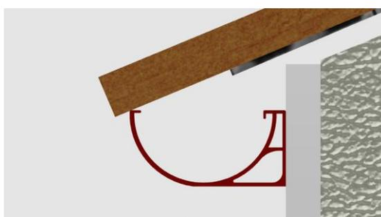
*A straight edge can be placed along the pitch of the roof to determine the position of the fascia bracket*
