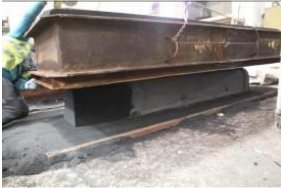
Mould box being fitted over core
