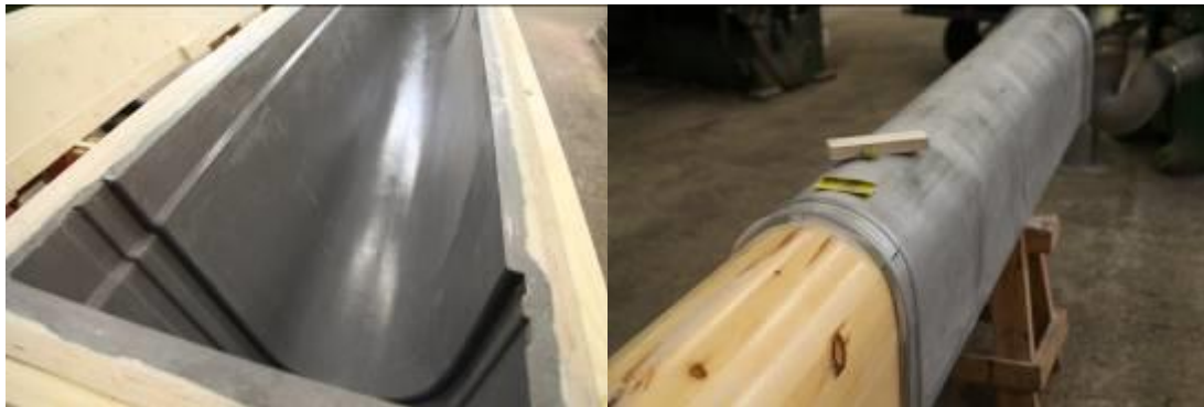
Resin core box made from slug
