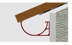
A straight edge can be placed along the pitch of the roof to determine the position of the fascia bracket
