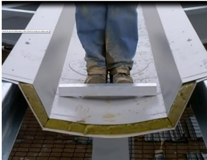
Thin gauge steel and the deflection
