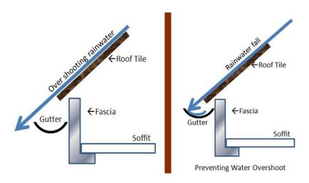
BS 5534:2014 (Slating and tiling for pitched roofs) states that roof tiling should project a minimum of 50mm from the vertical face of the fascia board. The projection should align with the centre line of the gutter and therefore this will establish the minimum width of gutter. However, there is no guidance as to the height of the gutter relative to the roof edge.
