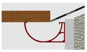
Use a spirit level against the lowest point of the roof tile to determine the position of the fascia bracket
